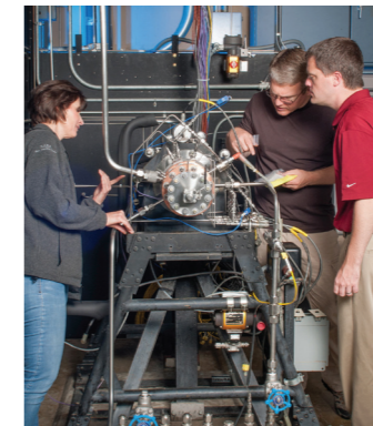
Below and right: Last year, engineers at NASA's Glenn Research Center in Cleveland, Ohio, successfully tested a 3D-printed rocket injector component using selective laser melting. The part withstood more than 9,000kg of thrust during hot-fire testing assessments
